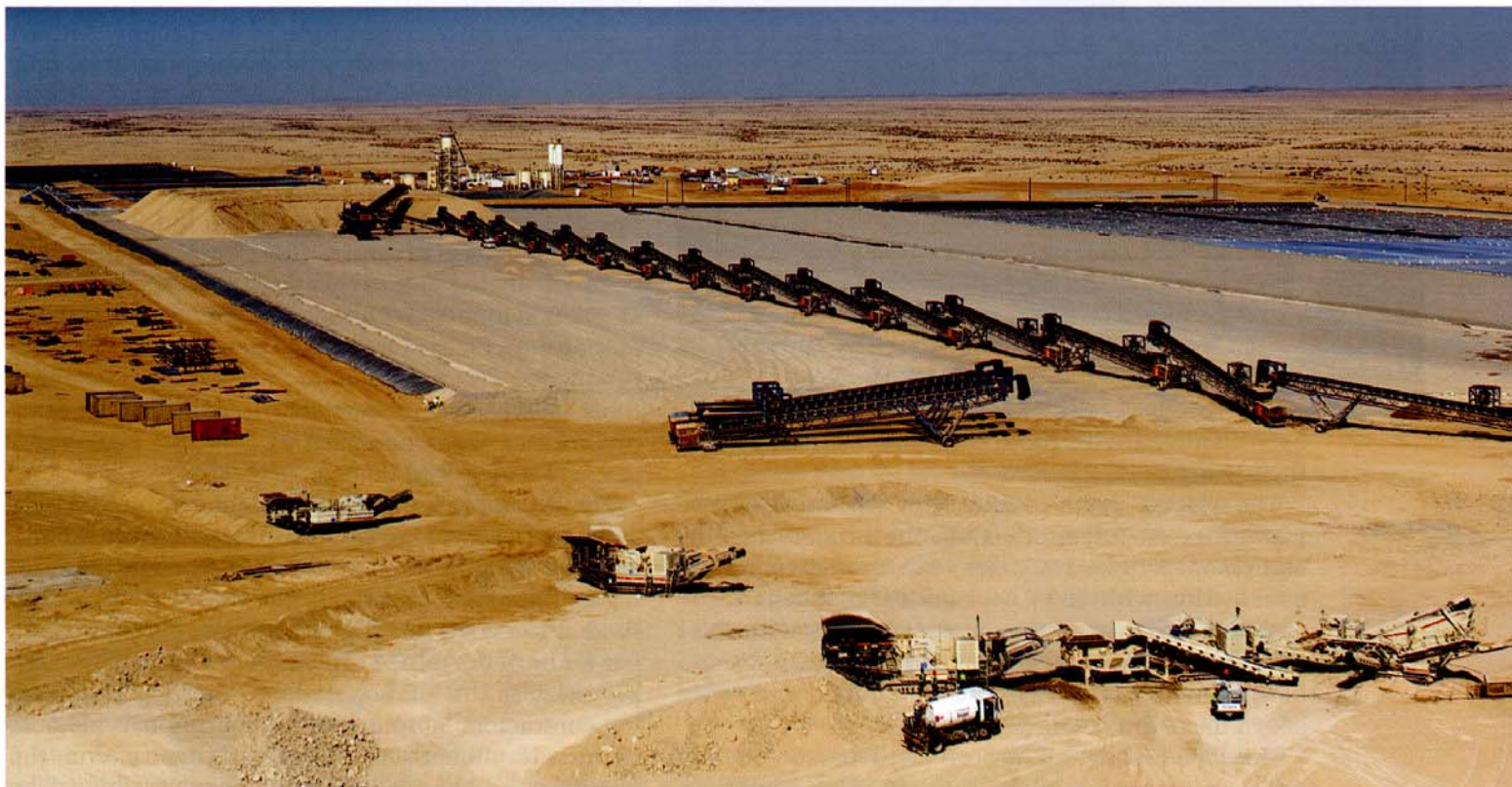
The MIDI plant consist of 10 cells x 300 000 t treating -38 mm crushed ore. The stacking rate is 9 000 t/day.
